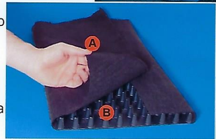
DrainStar Wall Drain 200 picture shows a two-part prefabricated soil sheet drain made up of polypropylene filter fabric (A) and polystyrene dimpled core (B).
